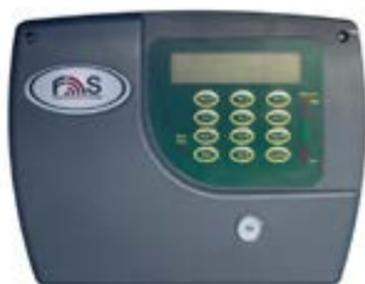
The Fuel Level Monitoring System is a 240v combined digital tank level indicator and bund and high-level alarm that is designed to provide both visual and audible alarms whenever a predetermined level in a storage tank is reached. The FMS gives a content readout in both litres and a percentage.
