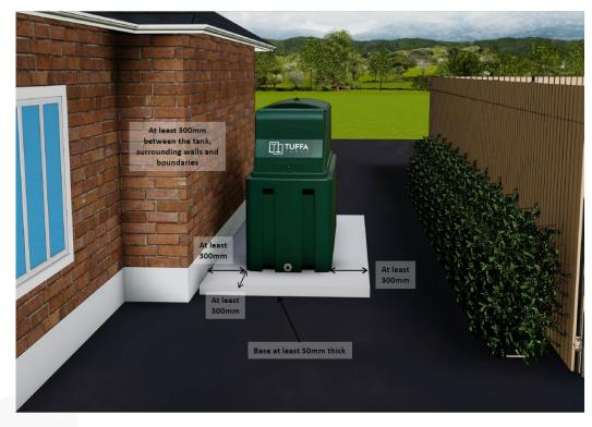
Typical external ½ Hour fire rated domestic Tuffa FP Tank installation:
